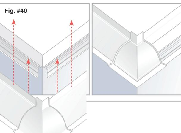
Cut the backing profile to length and mitre into the internal and external corners. A slight gap at the mitre is acceptable.
