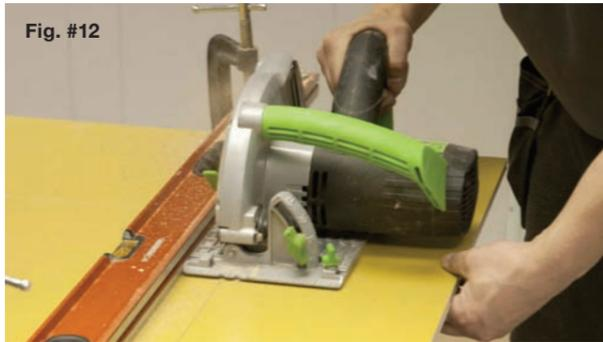
Panels can be cut using normal cutting tools. For best results the cutting action should be into the decorative face, so when using a jig-saw, the decorative laminate should be face down. The exception to this is when using a special "down cut" jig-saw blade, which should only be attempted if you are familiar with this tool (Fig #12).
