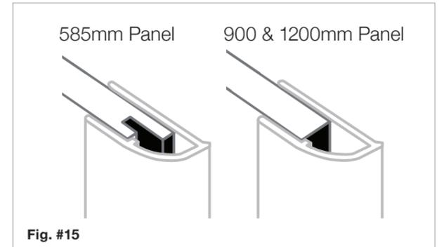
Apply masking tape to the curved face of the Transeal profile up to the bottom ridge. Starting with the middle profile (if any), lay a heavy line of Sealux-N in the channel formed between the strip upstand and the wall panel support leg.
